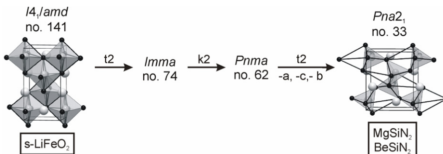
Figure 10. Group–subgroup scheme for s-LiFeO 2 and BeSiN 2 /MgSiN 2 . Both structures are presented in equivalent detail and the polyhedra of the partner structure are enhanced by thick black lines, respectively.
